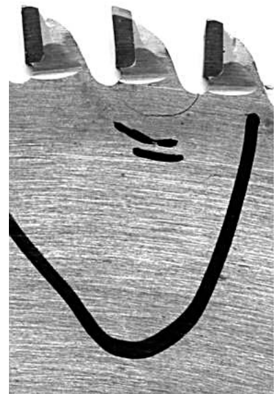
Cracked saw body
