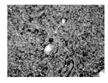
Standard flux at 50x magnification Large grains of foreign material
