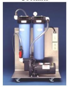
We now have a filter system that filters straight oil coolants. Above is our CP 2020 which filters tight oil coolant very well. It is also available as a wall mount unit.
