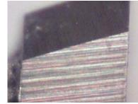
Nice even grind. No chips, no cracks, very slight hone on the edge. This was run and the customer was very pleased
