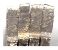
This is a 4x photo of four failed tips. You can see the grind marks on the steel in all four tips. You can also feel the grind marks by dragging your thumbnail over them. The grind marks can even be seen faintly with the naked eye in some places
