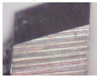
Good Grind Nice even grind. No chips, no cracks, very slight hone on the edge. This was run and the customer was very pleased
