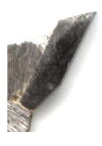
Above is a photo of a tip on the same saw. This tip did not come off. We ground the tip and carbide to expose the braze joint. There is very little braze alloy between the steel and the tip
