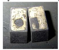
Here are two tips we pretinned and then etched with acid. The braze alloy flowed out nicely during pretinning and the tips looked good but there were huge holes in the middle where the braze alloy didn't stick to the carbide.
