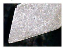
This is the tip before. I pushed the tip back and forth about an inch each way for 100 passes. Figure about half a minute for 100 passes.
