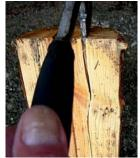
The piece of clear, straight grained wood on the left split much further with a single blow than the knotty piece on the right.
