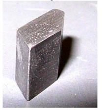
As near as I can tell you would need about 500 to 1,000 passes with a coarse hone to "sharpen" this tip. 500 passes would be about two and a half minutes. The four sides of a saw tip would mean about ten minutes per tip. You could sharpen a 24 tooth saw blade in just four hours with a coarse diamond hone.
