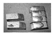
The left column shows the face of the tips with a thick layer of braze alloy all over them. The bottom tip has piece of steel slag. This is going to cost a fortune to grind unless you just throw the tips away. The right hand column shows tips with globs of braze alloy on them. This is poor bonding and means the tips are more likely to come off or break.
