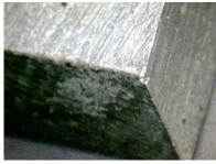
This is the tip after 100 passes on each of the three sides shown. The light patch in the dark area is a dip in the surface that I didn't get down to.
