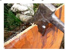
When you hit piece of plywood you can initiate a crack but it doesn't go anywhere. You have to keep cutting and cutting in the same place until you gnaw your way through it.
