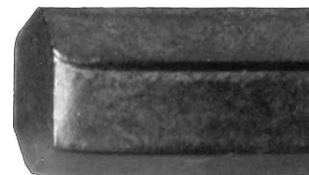
Competitor: Tip bent by cutting process
