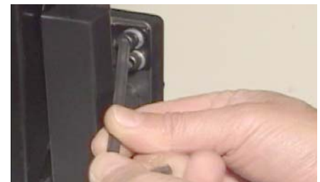
Ball end tool provides continuous rotation
