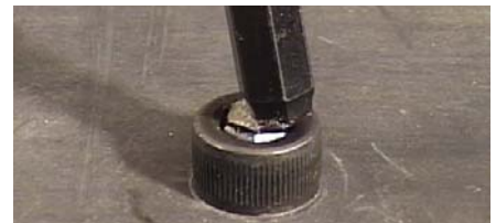
Competitor tool: Thin neck size risks breakage
