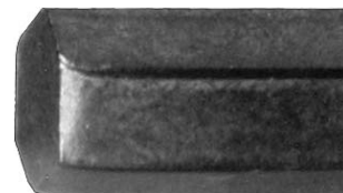
Competitor: Tip bent by cutting process
