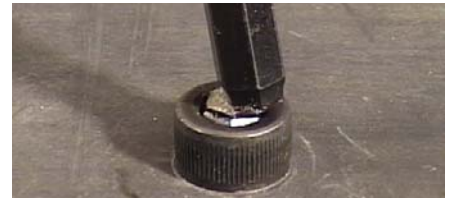
Competitor tool: Thin neck size risks breakage
