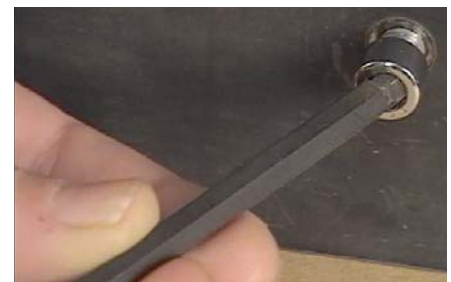
Ball end tool provides continuous rotation
