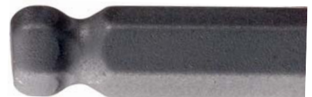
Competitor tool: Imprecise machining causes undersized tips
