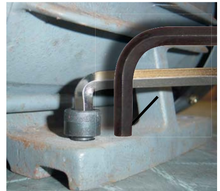
Not enough overhead clearance for standard hex key
