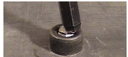
Competitor tool: Thin neck size risks breakage
