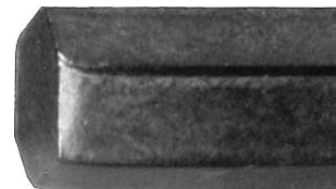
Competitor: Tip bent by cutting process
