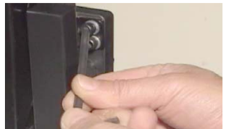
Ball end tool provides continuous rotation
