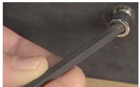
Ball end tool provides continuous rotation
