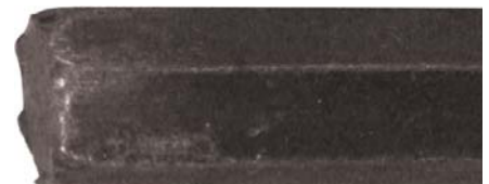
Competitor: Tip with lips will not seat to full depth
