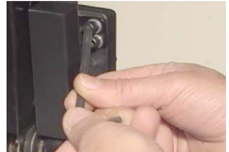
Ball end tool provides continuous rotation
