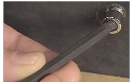
Ball end tool provides continuous rotation
