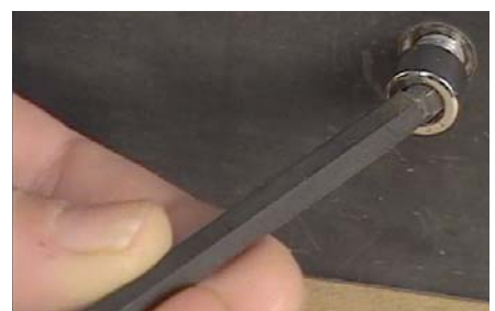
Ball end tool provides continuous rotation
