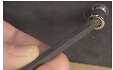
Ball end tool provides continuous rotation
