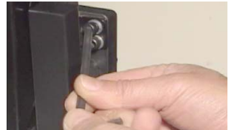
Ball end tool provides continuous rotation
