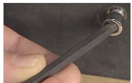
Ball end tool provides continuous rotation
