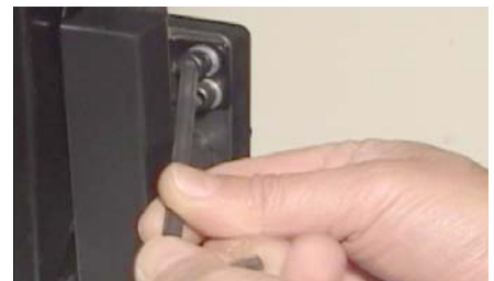
Ball end tool provides continuous rotation
