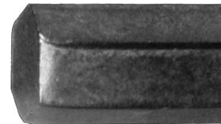
Competitor: Tip bent by cutting process
