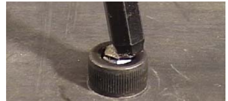
Competitor tool: Thin neck size risks breakage
