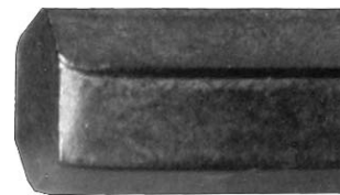
Competitor: Tip bent by cutting process
