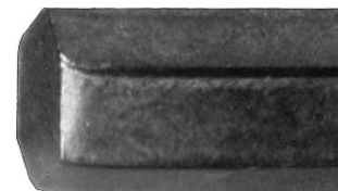
Competitor: Tip bent by cutting process
