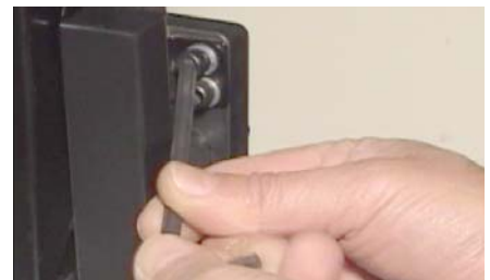
Ball end tool provides continuous rotation
