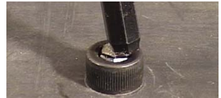
Competitor tool: Thin neck size risks breakage
