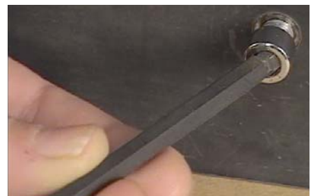
Ball end tool provides continuous rotation
