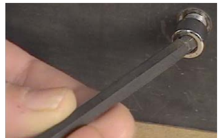
Ball end tool provides continuous rotation
