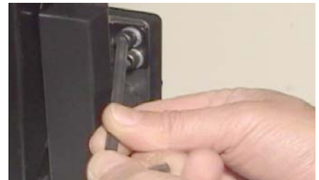
Ball end tool provides continuous rotation
