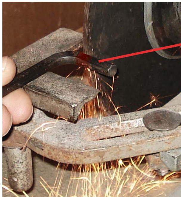
Cutting a standard hex key is an inadequate substitute for a Bondhus Stubby tool.
