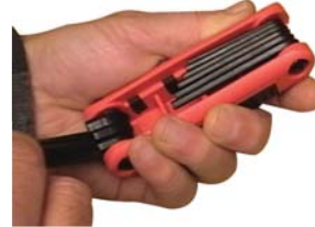
1) First layer is folded out of the way.
