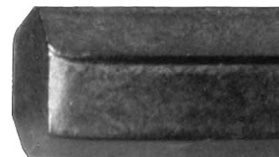
Competitor: Tip bent by cutting process
