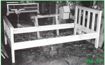
Check that the bed is square and measure the distance between the side rails. It should be about 930 mm. Cut the six slats (E) using the Workcentre in the crosscut mode (**Fig. 20**).
