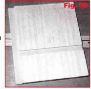
Cut the dividers ( $\frac{d}{d}$ ) to fit into 4mm deep rebates in the top and the shelf. Position them 202mm from the sides to create a 202 x 61mm opening for the drawers to fit into.
