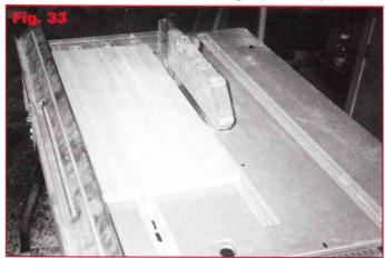
Cut the writing slope edges (N & O) to size from jarrah and mitre the corners with the protractor fixed at 45 degrees.
