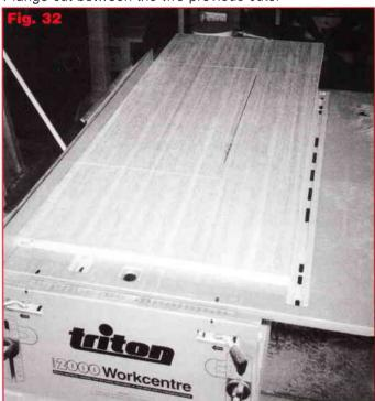
To do this, hold the desk top against the fence, but angled above the saw blade and start the saw. Slowly lower the desk top onto the saw blade so the cut begins in the middle of the piece of wood (**Fig. 32**). Don't saw right up to the cuts, stop short and remove the desk top.
