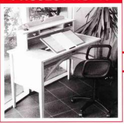
Tassie oak or any other suitable hardwood can be used for the desk frame. The panels are veneered board and the dark timber highlights are made from jarrah. The drawer fronts feature decorative finger joints. Of course, the desk top can be made in one piece and the writing slope omitted if so desired.
