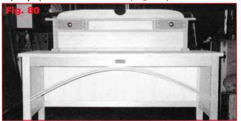
Mark the desk under the centre of the base feet at each end. A single 8G x 30 mm screw at each end, screwed from underneath the desk into the centre of the side base feet will hold the shelf unit in place.
