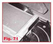
Attach the base feet by standing the shelf unit upside down and drilling, gluing and screwing from underneath.
