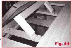
A small wedge (U) is glued to the top of the push rail and rests against the closed trestle. Its job is to push the trestle and writing slope upwards when the push rail is pushed in. It needs to lift the writing slope high enough so the rear of it can be lifted with the finger lifter slot.
