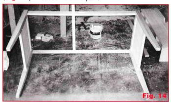
The stretcher rails have 4 notches in them to receive the trestle legs and support the writing slope when it is in the raised position.
