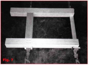
Check that everything is square by measuring the diagonals. Adjust the clamps until both measurements are identical.
