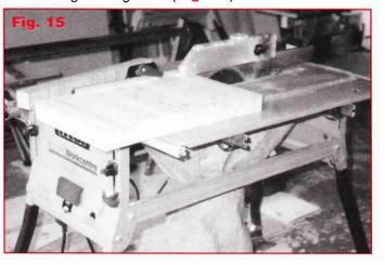
Trim strips of blocks by setting the rip fence to, say 44mm, then machining one side of each strip first. Then set the fence to 42mm and machine the other side, to provide 12 strips of blocks 42mm wide and 45mm high.
