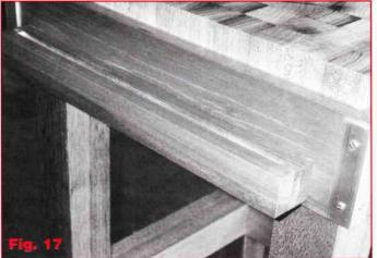
Mount the knife rack with three 8G x 30 mm screws driven from behind one of the sides, which will also conceal the screw heads.
