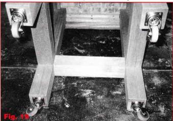
Chamfer the base of each leg slightly by hand sanding the edge at a  $45^{\circ}$  angle.
